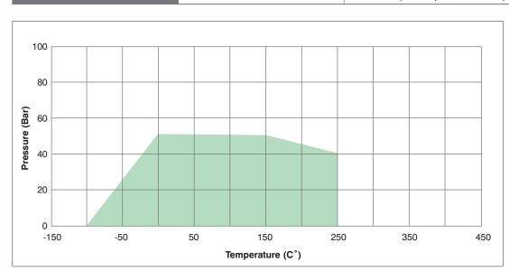
Pressure x Temperature curve indicates the service limits considering the simultaneous influence of temperature and pressure. The green area represents the normal service limits for non-critical media (excluding steam) for 2mm thick material.
